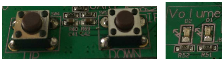
Figure16. Volume control button switch and indicate LED
